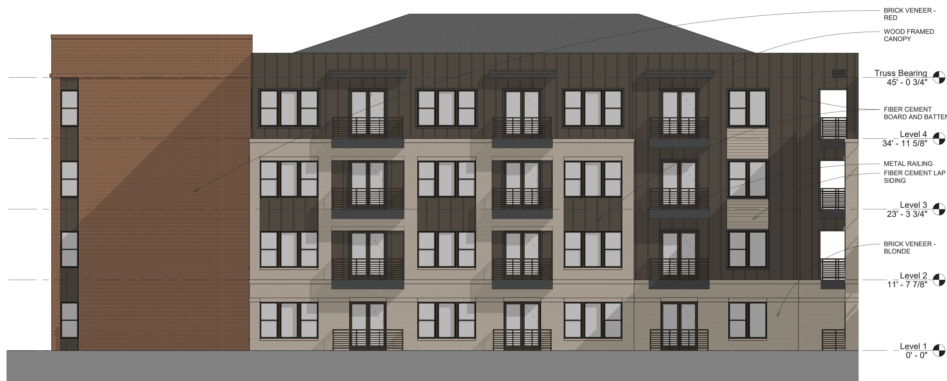
② Overall North Elevation - Part 2 1/8" = 1'-0"
